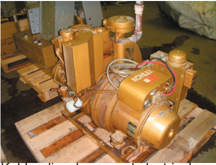
Kohler diesel powered electrical power plants. 4 KVA, approx. 1100 hrs. Breaker panels. Electric start.
